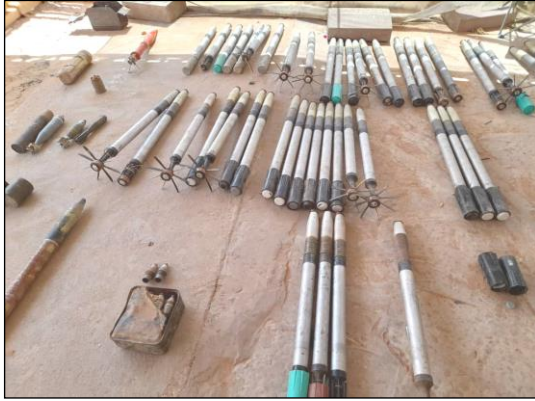
Unguided S-5 air-to-ground rockets, mortar shells and a box with S-5 fuses (bottom left)
