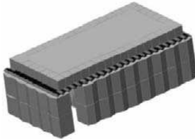
Figure 8-41. Artist sketch of completed bunker (app. 36' long x 18' wide x 12' high)
