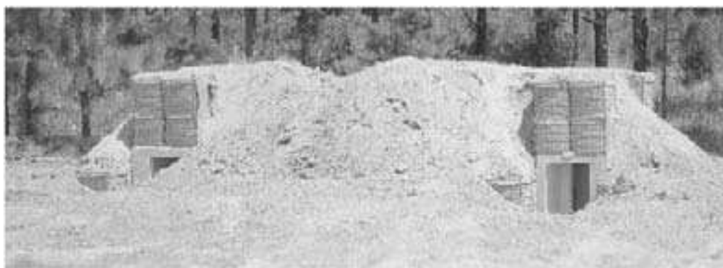
Figure 8-39. Post-test photo of simulated 122 mm rocket over roof of cut and cover configuration of modular concrete bunker with 4' of soil cover: No damage inside.
