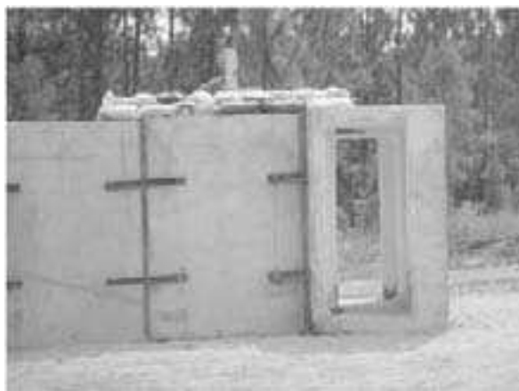
(a) Pre-test with mortar on top of 2 layers of sandbags
