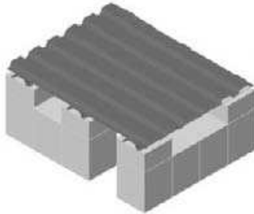
Figure 8-72. Artist concept of optional sheet pile roof.
