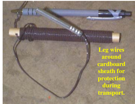
Figure 1.5. Typical Electrical Blasting Cap
