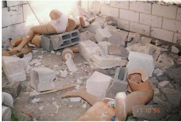
Figure 3.17. CMU Debris Impact on Mannequins
