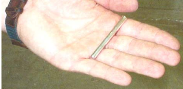
Figure 1.6. Typical Non-electrical Blasting Cap
