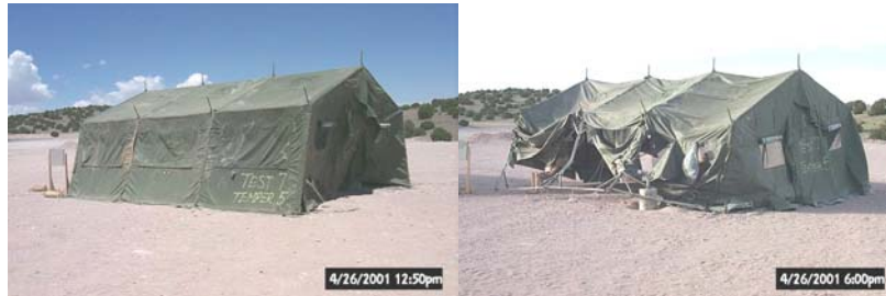
Figure A4.37. RODS Pre and Post Test of TEMPER Tent
