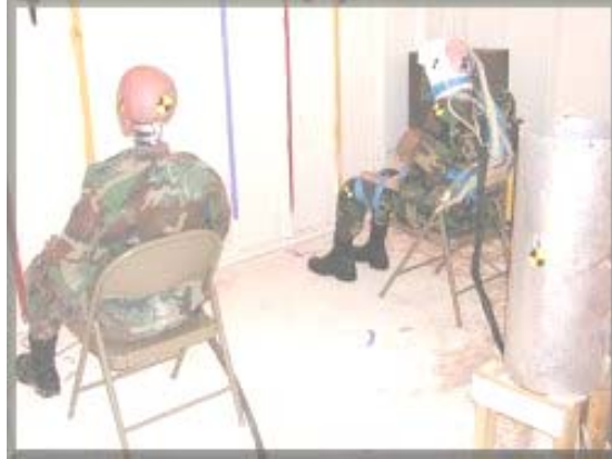
Figure A4.13. BAIT Pre-test SEA Hut Pre-test Anthropomorphic and Cadaver Setup Inside a SEA Hut
