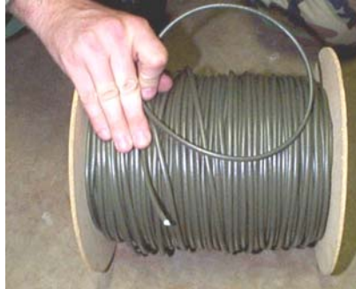
Figure 1.7. Typical Roll of Military Det Cord
