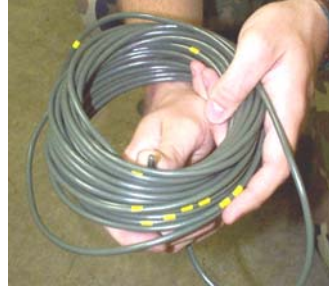
Figure 1.4. Roll of M700 Time Fuze
