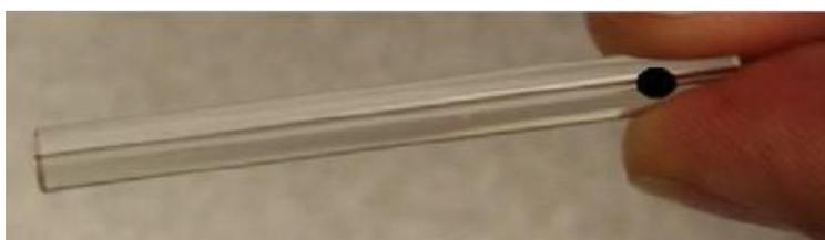
**Figura 23 – FIDO X3 *sensing element***
