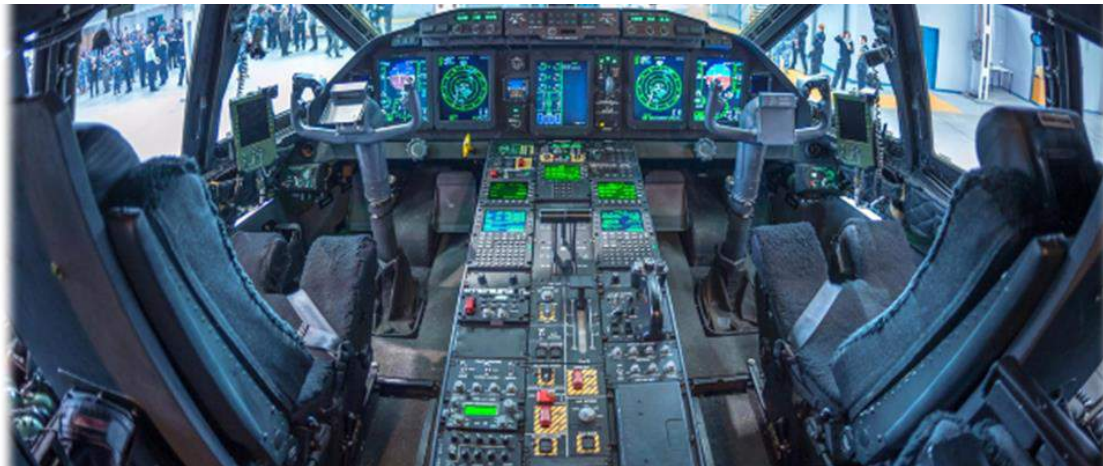
State-of-the-art avionics compliant with Next Gen Air Traffic Control requirements, including FANS 1/A+ datalink, TCAS 7.1, ILS Cat.II, enhanced video TAWS
