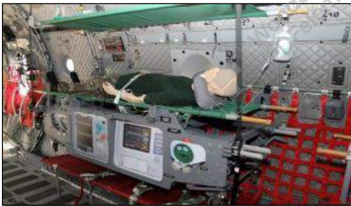
C-27J - Example of medical arrangement and equipment for the transport of a patient in critical condition requiring special medical care
